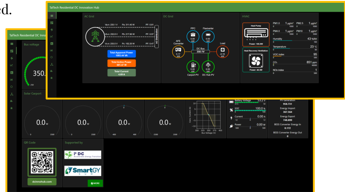
Fig: DC Microgrid monitoring platform
